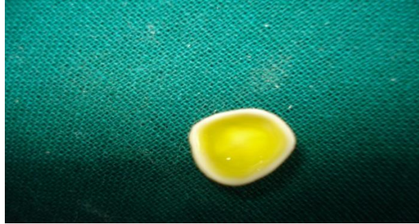
Figure 6: Hydrofluoric acid etchant &etchant applied onto the Zirconia Coping.
