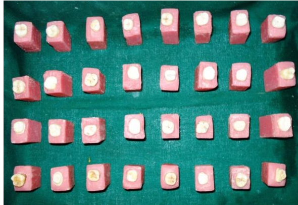
Figure 1 : Mounted natural human molar teeth embedded in autopolymerising resin
