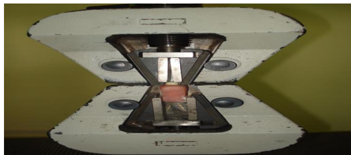
Figure 9: The Zirconium oxide ceramic copings subjected to tensile forces in the Universal Testing Machine
