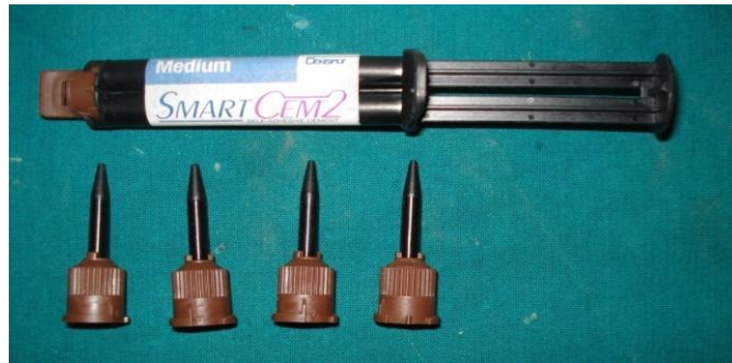
Figure 7: Smart Cem 2 resin cement used for cementing the specimens
